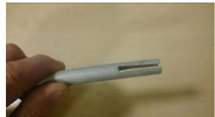
Once the reel drum had been taken apart the damaged section of cable was cut out, but to re-terminate the cable it had to be connected to the existing crimp pins used on the slip ring assembly. In the picture on the right the damaged cable is just out of shot.
