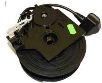
The vacuum cleaner was then fully reassembled and tested and now with an undamaged power cable is once again safe to use. This repair is a good example of the efforts required to repair a product that is actually not designed for disassembly and repair.
