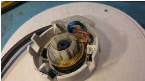
The cable was cut about 20mm from the slip ring crimp pins and an in-line solder joint was made up and covered with heat-shrink sleeving. The in-line joints are not subject to stress because they are downstream from the cable clamp.
