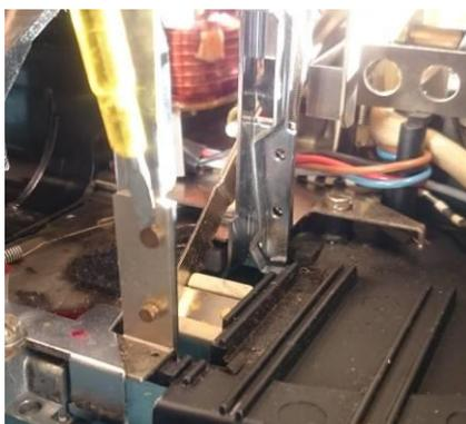
The picture shows the two peened rivets on the other side of the slide frame which are still in place, as indicated by the yellow sleeved screw driver blade.
