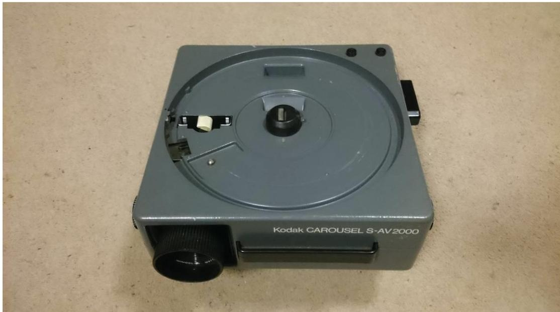
**The fault symptoms** on this projector were complex in as much as the mechanism would get completely confused. Sometimes it placed two slides in one carousel slot. Other times it would try and index the carousel with a slide half in and half out which would cause a jam and put lots of strain on the drive motor inside.
