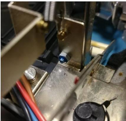
To ensure that the M2.5 nut and bolt won't come undo Loctite 243 (blue) was used to lock the nut threads in place. This should ensure a long lasting repair but if really necessary the nut can be removed by unlocking the Loctite with a heat gun.
