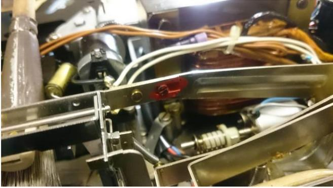
Close inspection showed that the slides were not being lifted fully out of the projector before the carousel was indexed to the next slide. This was traced to the original slide arm which whilst having been bent straight was now not lifting the slides correctly. This was corrected by adjusting the offset cam on the slide arm (red caped screw). This adjustment was very sensitive and took several attempts to get it right.
